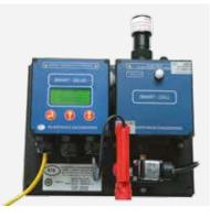
**AUTOCLEAN** > The autoclean option has been designed to ensure that the measuring cell glasstube is kept free from fouling. Cell fouling is recognised as a leading cause of monitor malfunction. Fitting the Autoclean removes the need for the ship's crew to remember to clean the cell manually.
