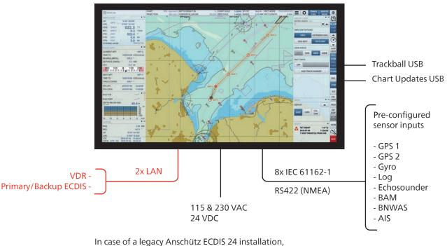
In case of a legacy Anschütz ECDIS 24 installation, the magicplex can still be used and easily connected via LAN to the new panel-pc.
